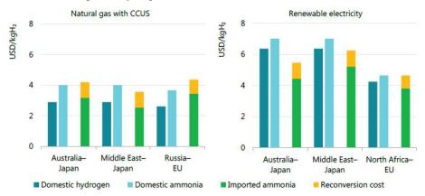
Figure 4 Comparison of delivered hydrogen costs for domestically produced and imported hydrogen for selected trade routes in 2030
